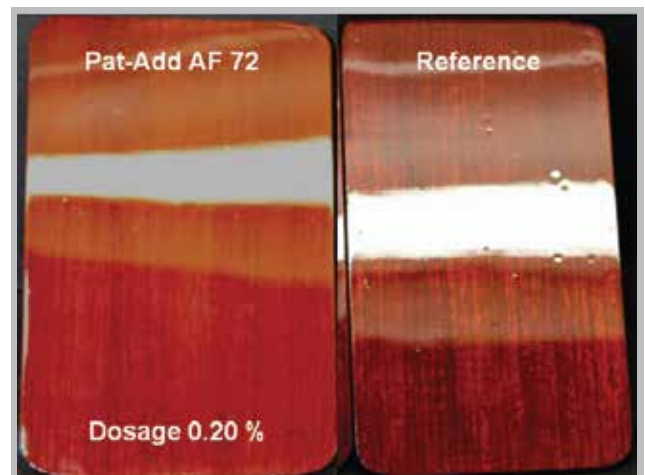
Spray Application of 2KPU Clear on Wood Panels
